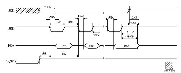
Figure 11-4 Serial Access Cycle after Read
