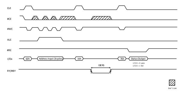
Figure 9-23 Block Erase Operation
