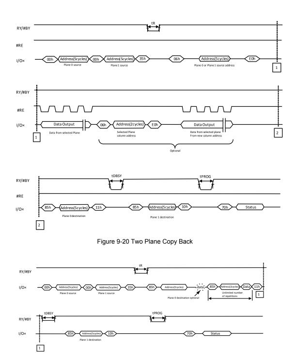
Figure 9-21 Two Plane Copy Back with Random Data Input
