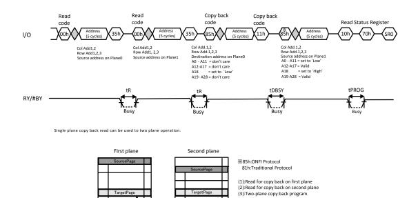
Figure 9-22 Two Plane Program for copy back
