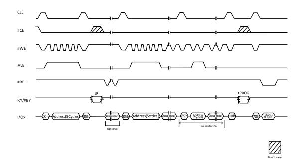
Figure 9-19 Copy Back Operation with Random Data Input
