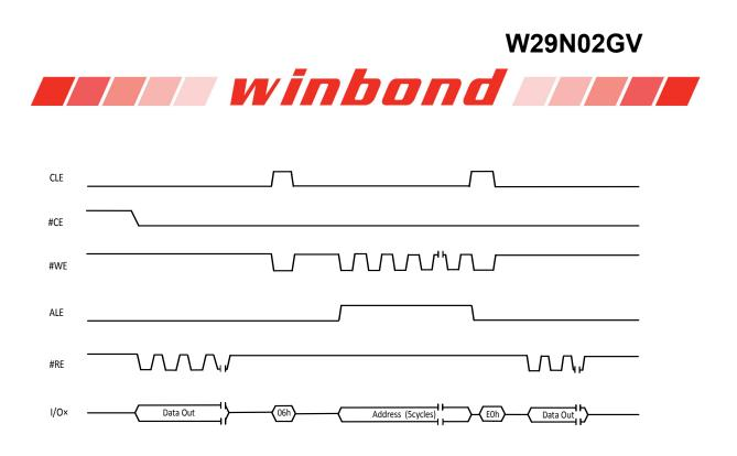
Figure 9-7 Two Plane Random Data Read (06h-E0h) Operation
