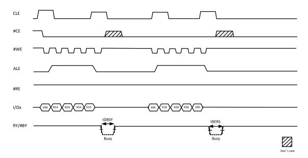
Figure 9-24 Two Plane Block Erase Operation
