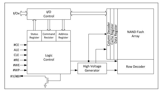
Figure 5-1 NAND Flash Memory Block Diagram
