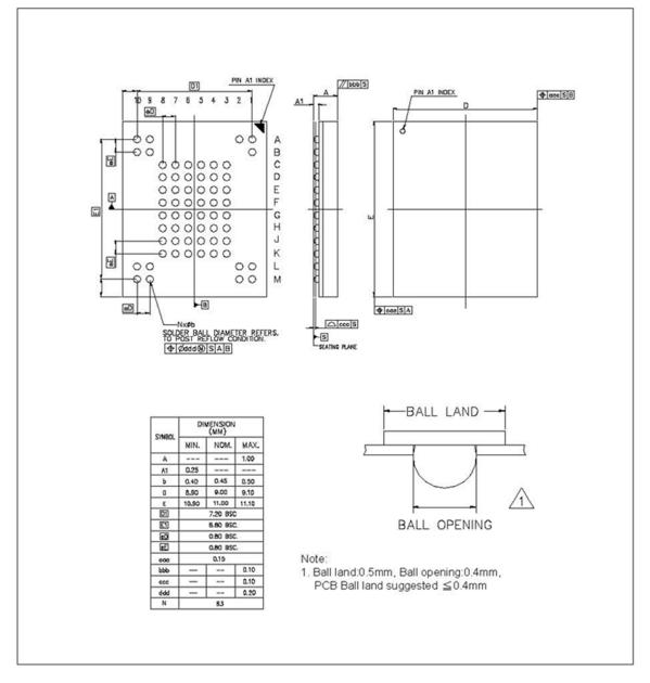
Figure 13-2 Fine-Pitch Ball Grid Array 63-Ball
