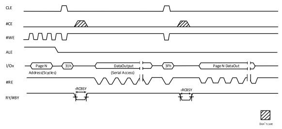
Figure 9-4 Last Address Cache Read Operation
