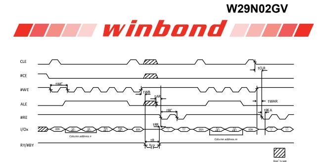
Figure 11-9 Random Data Output Operation
