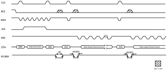
Figure 9-2 Sequential Cache Read Operations
