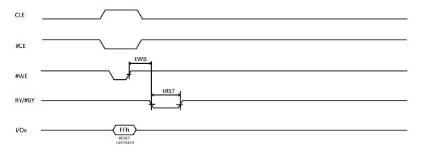
Figure 9-25 Reset Operation
