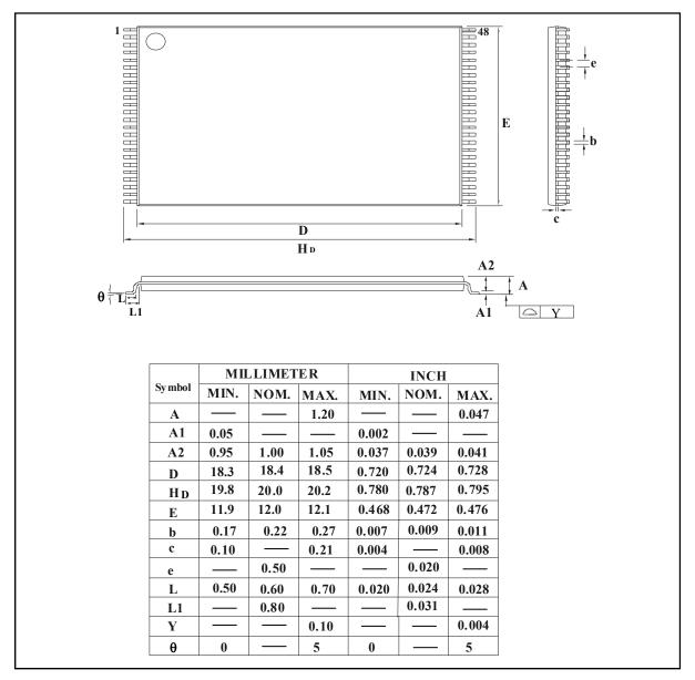
Figure 13-1 TSOP 48-PIN 12X20mm
