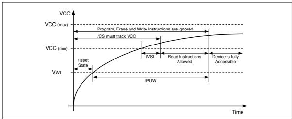
Figure 58a. Power-up Timing and Voltage Levels
