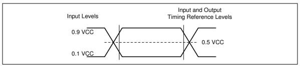
Figure 59. AC Measurement I/O Waveform
