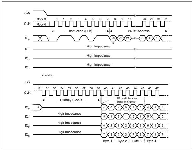
Figure 20. Fast Read Quad Output Instruction
