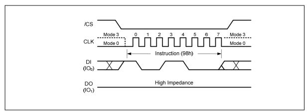
Figure 57. Global Block Unlock Instruction for SPI Mode
