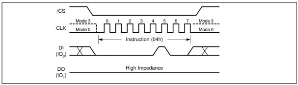
Figure 7. Write Disable Instruction for SPI Mode
