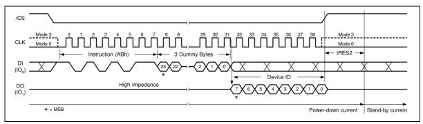
Figure 38c. Release Power-down / Device ID Instruction
