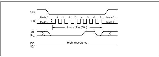
Figure 5. Write Enable Instruction for SPI Mode
