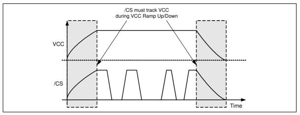
Figure 58b. Power-up, Power-Down Requirement
