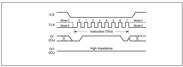
Figure 56. Global Block Lock Instruction for SPI Mode
